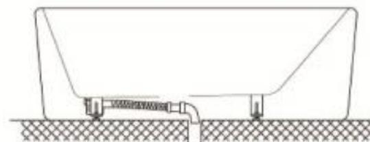
**4. Fill the tub with water in order to test it for leaks**
