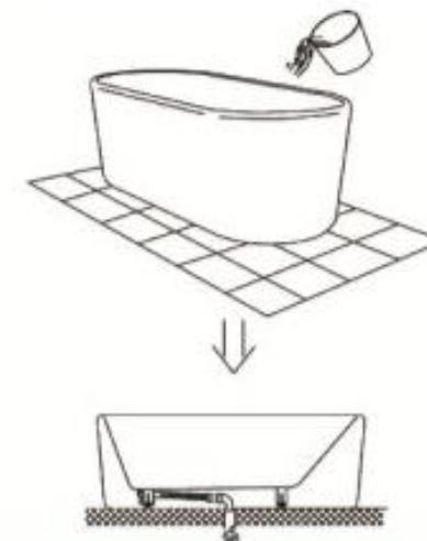
**WARNING!** To avoid the bath to be scratched - put it on a soft material during the installation (carpet, construction cardboard).
